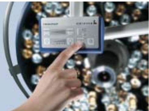
Fig. 2 : Ergonomic, intuitive adjustment directly on the lighting unit itself with symbols for turning the light on and off or adjusting parameters like the light field, lighting intensity, and colour temperatures
