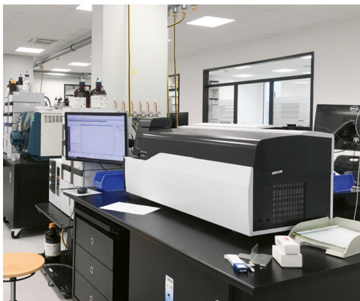
Currently used by the lab for forensic and clinical purposes, LC-MS primarily detects active ingredients in medication, hormones and drugs
